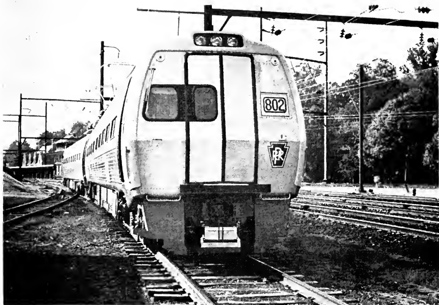
Fig. 3—Stainless steel Metroliners are 85 ft long.
